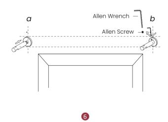
6. Install the rod onto the bracket (if using rings, add rings at the same time).
