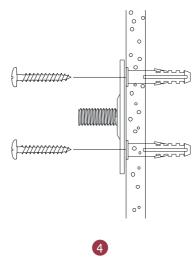
4.Install the bracket fixing.
